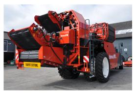
The 9th model of the successful R3060 series was introduced during the Sima fair earlier this year. Potato Europe will be the first opportunity to see the RF3060 in action. The harvester is equipped with the revolutionary Flexyclean® cleaning unit, a patented variable bypass system in combination with axial rollers, which responds perfectly to any conditions. The RF3060 enables you to quickly accommodate changing
