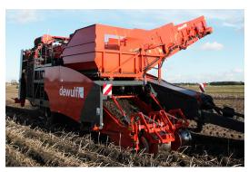
This side-mounted harvester is the absolute champion in the 2-row trailed potato harvester segment. No other trailed potato harvester achieves the capacity of the R2060. Cleaning is performed by three sieving belts, a bottom hedgehog belt, a cleaning module and a top hedgehog belt. The R2060 has the largest tyre size in its class, keeping ground pressure to an absolute minimum. The harvester offers unloading
