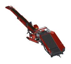
The Miedema MHC 241 SZ 12 creates the total solution for buffering, sorting, cleaning, inspecting and transporting your product. This combi is a large capacity machine that provides cleaning by means of 12 coil rollers with Smart-Pin.
