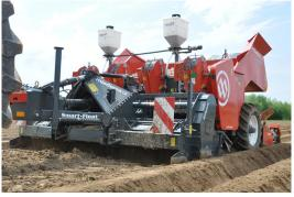
The CP cup planter is a multifunctional, large capacity potato planter which has proved its qualities time and again in the field. The CP 42P offers integrated tillage and is equipped with Smart-Float, a unique cultivator depth control system. Thanks to the low-pressure tyres and the ridging hood with MR-control, perfectly shaped ridges are standard here too. The latest innovation, Erosion-Stop, gives a remarkable boost to the potato grower's yield.
