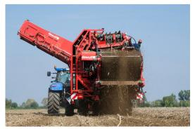
For this trade fair, the side-mounted harvester RJA2060 is equipped with driven discs that provide an absolute advantage in the event of wet conditions. Cleaning is performed via 3 sieving belts, a hedgehog belt and an easy-clean module. Remaining clods are removed from the machine at the top by means of a flat hedgehog unit with a 4-row drive away belt. The R2060 has the largest tyre size in its class, keeping ground pressure
