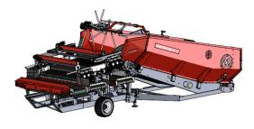
With the MH 201, Miedema has been able to introduce a receiving hopper to the market, which has more volume and as a result a higher buffer capacity. The bunker floor has a length of 5.7 metres and is therefore 110 cm longer than its smaller sibling, the MH 200. The first 110 cm of the bunker floor is flat, as a result of which tipper trailers with a larger projection can also be easily used. The flat bunker floor prevents any rolling
