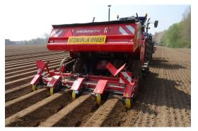
The CP cup planter is a multifunctional, large capacity potato planter which has proved its qualities time and again in the field. Optionally, a Smart-Float combination can be selected, which enables planting and cultivation in a single operation. The latest innovation, Erosion-Stop, gives a remarkable boost to the potato grower's yield. This hydraulically driven, patented machine is installed on the ridging hood and builds up
