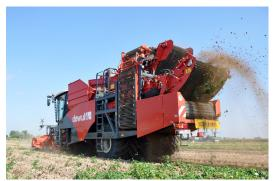
This 2-row self-propelled harvester is equipped with the revolutionary Flexyclean® cleaning unit, a patented variable bypass system in combination with axial rollers, which responds perfectly to any conditions. The RF3060 enables you to quickly accommodate changing conditions during harvesting and adapt the cleaning intensity without having to shift the harvester's centre of gravity. Thanks to Flexyclean®, it is possible to clean the
