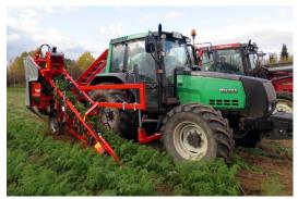
The Dewulf P3K is equipped with a discharge elevator that ensures maximum capacity. The isolated cross conveyor below the cutters safeguards a minimum falling height of the product and an optimal filling of the 3-part discharge elevator. The top lifting harvester with 3-point linkage has a new maintenance-free 'Gearbox Drive'. As a result, the capacity is increased considerably, while a high-quality end product is guaranteed. From now on, the
