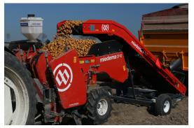
The new Miedema ME 60 Planter Filler is a conveyor belt with a length of 6 metres that seamlessly connects to the tipper trailer. With a capacity of no less than 100 tonnes/hour, the planting machines are filled with remarkable speed. The steplessly adjustable speed of the trough belts ensures a thick product flow. Due to the hydraulically rotating transport frame, the pivoting of the filling belt is extremely comfortable. Its versatility
