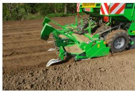
A cultivating tine is mounted in front of the shovels, in order to have sufficient loose soil and to improve the infiltration of water between the ridges. The cultivating tine is adjustable in depth. The frequency of the up and down movement of the shovels is also adjustable so that the distance between the ditches can be adapted as a function of the soil and the slope, This is done via the display of the planting machine.
