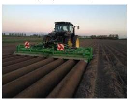
With a working width of up to six meters, the new folding AVR GE-Force plows major surfaces in a single motion.
