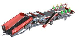
The Miedema MHC forms your total solution for buffering, sorting, cleaning, inspecting and transporting your product. This combi is a large capacity machine that provides cleaning with a double stone and clod separator. Thanks to the integrated discharge conveyor you are able to fill the store, crates or lorry with perfectly clean product.
