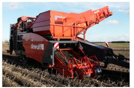
This offset harvester is a true high capacity machine in the 2-row trailed potato harvester segment and is available in six different versions. The RA2060 makes use of three sieving conveyors, a lower hedgehog unit, a cleaning unit (axial, easy-clean or a sieving module) and an upper hedgehog unit. The R2060 has the largest tyre size in its class, keeping ground pressure to an absolute minimum. The harvester is fitted standard
