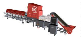
The Miedema Smart Grader has a unique singling system with vibrating axial rollers. During operation the tubers are scanned on all sides and registered by smart cameras and sensors, after which air nozzles blast the product to the right exit. This results in very accurate sorting by size, shape and quality, and thus in a more homogeneous end product and a higher market value. Thanks to its modular construction, the Smart Grader is
