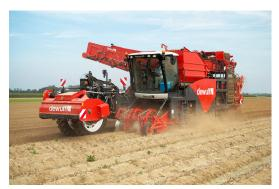
Thanks to a quarter century of unmistakable craftsmanship, the R3060 has become a pioneer in the 2-row self-propelled sieving harvester segment. Owing to its modular construction, the harvester is available in no fewer than nine different versions. The RA3060 will be on display throughout Potato Europe. This harvester is equipped with three sieving conveyors, a lower hedgehog unit, a cleaning unit (axial, easy-clean
