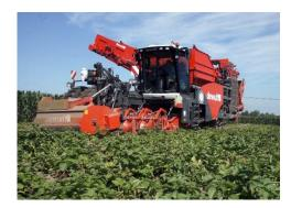
With the 5<sup>th</sup> generation of the 3-wheeled 2-row self-propelled potato harvesters, the R3060 had a complete redesign with a focus on the driver. No less than 8 different harvester versions ensure a fully customized machine. During Potato Europe, the RA3060 will be demonstrated. This harvester is equipped with 3 webs, 2 hedgehog belts and axial rollers. Thanks to a new set of instruments: harvesting display, traction display and joystick, harvesting was never before so easy.
