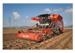
With the facelift of the Kwatro, Dewulf paid extra attention on the ergonomics for the driver and is the harvester your guarantee in all conditions. With the new Claas-cabin and set of instruments, on the same base of the R3060, Dewulf draws the line in comfort and ease of use. Larger driving wheels of the tracks ensure less soil pressure and less wear as big advantage. A large bunker of 17,5m<sup>3</sup> gives the guarantee of maximum capacity.
