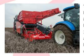
This sublime offset trailed potato harvester is equipped with a harvesting unit driven discs instead of diabolo rollers and an integrated haulm chopper. Thanks to this unit, it's possible to harvest under all circumstances in one time. Cleaning is based on 3 sieving webs, lower hedgehog belt followed by axial rollers and a flat upper hedgehog belt with 4-row finger system. The R2060 has the biggest wheel tires in its segment and is equipped with unloading on the move as a standard.
