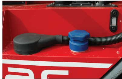
Excellent accessibility to the 30 litres AdBlue tank. The tank is integrated into the oil tank and can't be mistaken with its blue filler cap.
