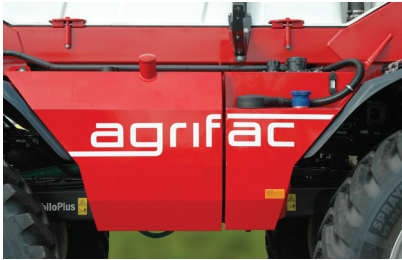
Excellent accessibility to the 30 litres AdBlue tank. The tank is integrated into the oil tank and can't be mistaken with its blue filler cap.
