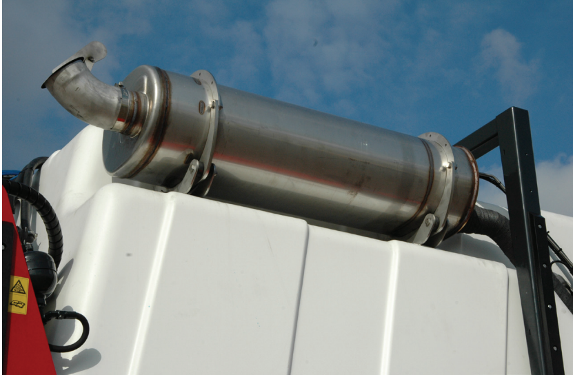
The maintenance free SCR-muffler is fitted above the main tank.
