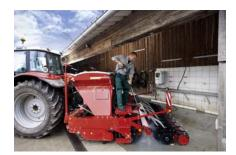
Models HD 7/16 ST, HD 9/18 ST and HD 13/12 ST are available in more than 100 versions and are used in agriculture, the crafts and trades, industry and municipalities. They operate with a maximum pressure of 180 bar and a water flow rate of up to 1,300 litres/hour.
